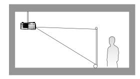
After turning on the projector, go to **Advanced** menu - **Installation Menu** > **Projector Position** and press **◄/▶** to select a setting.
