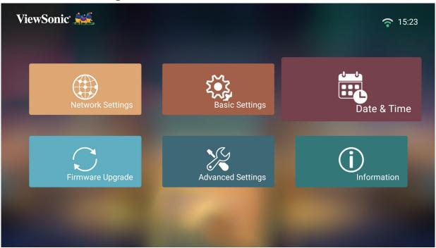
2. Use the **Up** and **Down** buttons to select the desired option and press **OK**. Then use the **Left** and **Right** buttons to make adjustments or selections.
