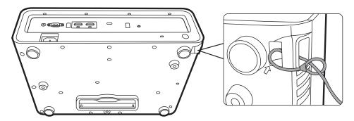
**NOTE:** The security slot can also be used as a safety anchor if the projector is mounted to the ceiling.
