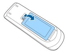
Remove the old batteries, if necessary.
