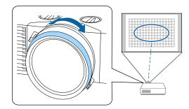
Adjust the corner focus while looking at the four corners of the projection screen.
