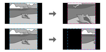
• **Full Display** to adjust the image to the projector's screen size as you scale the image.
