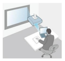
Turning off simple AP mode lets you connect to smartphones, tablets, or computers over a wireless network access point. Select this mode when connecting using Epson iProjection's Advanced Connection Mode (EB-L690SE/EB-L695SE).
