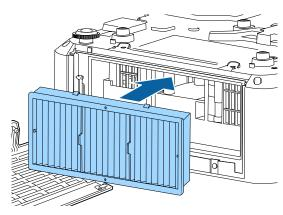
**9** Close the air filter cover and tighten the screws.
