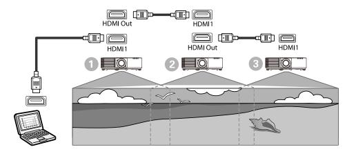
Connect the projector to the computer using the HDMI cable, and then connect the HDMI1 port and HDMI Out port of the projectors using the HDMI cable.
