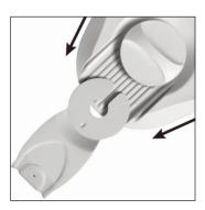
Speed-Lock<sup>™</sup> Mounting System Just slide the speaker onto the bracket until you hear the "click." The Speed-Lock Mounting System ensures easy, safe one-handed installations and no-slip setting of the speaker angle.
