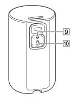
**9** Mounting hole for the general speaker stand 10 Wall mounting hole
