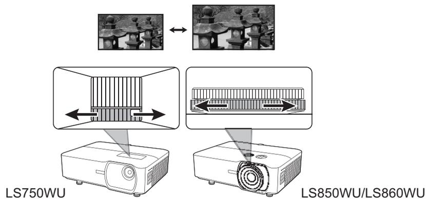
To improve the clarity of the image, rotate the Focus Ring.
