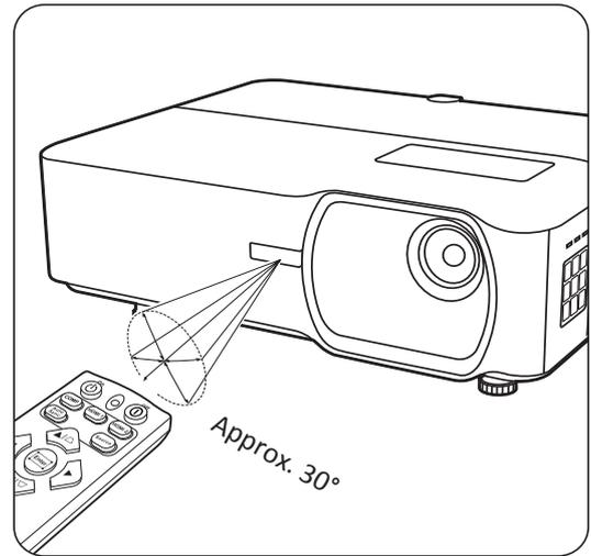
**NOTE:** Refer to the illustration for the location of the infrared (IR) remote control sensor(s).
