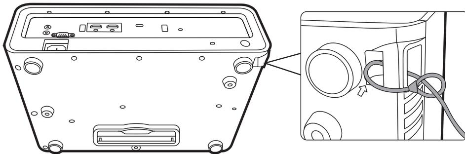
**NOTE:** The security slot can also be used as a safety anchor if the projector is mounted to the ceiling.
